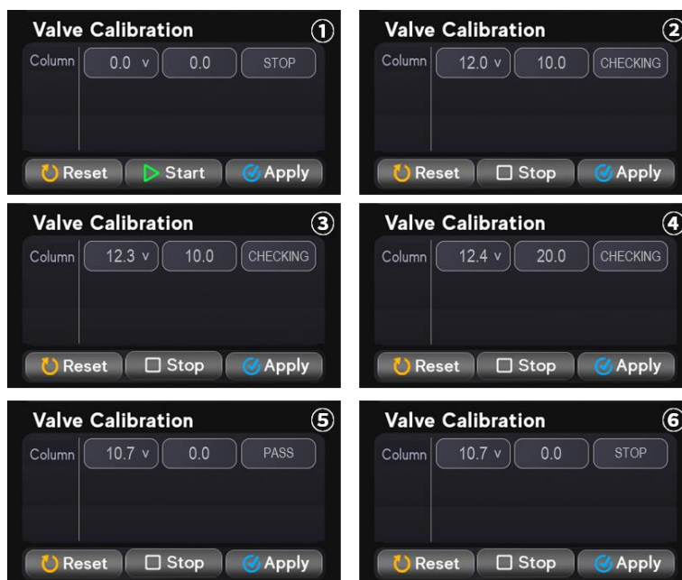
Figure 9. Valve calibration procedure for packed inlet
