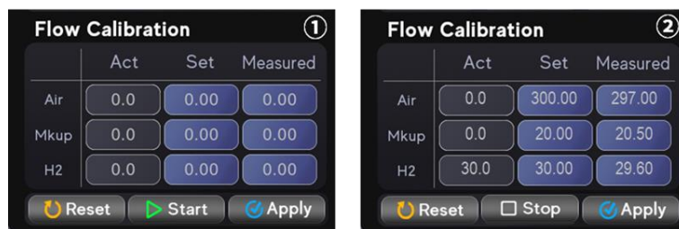
Figure 13. Flow calibration procedure for FID
