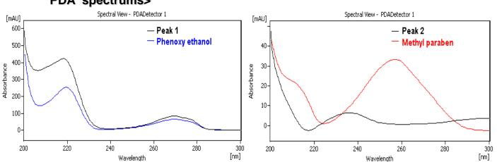
Peak 1 and Phenoxy ethanol are same spectrum pattern each so it can be recognized as same components,
